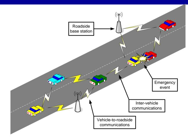
Vehicle to Vehicle communication (V2V), Vehicle to Infrastructure communication (V2I), Vehicle to Pedestrian communication (V2P)
